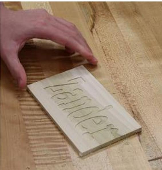
Example of 2D Milling (routing)
